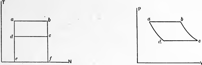
Figs. 162 and 163. Arts. 368, 406, 603. — Specific Volumes by Clapeyron's Method.
